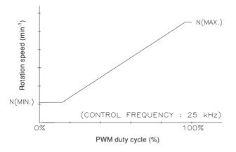
Fig. 4: Example of PWM specifications
